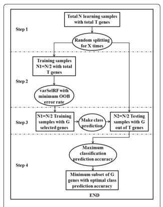
Figure 1 Flowchart of the Splitting Random Forest (SRF) Algorithm.
